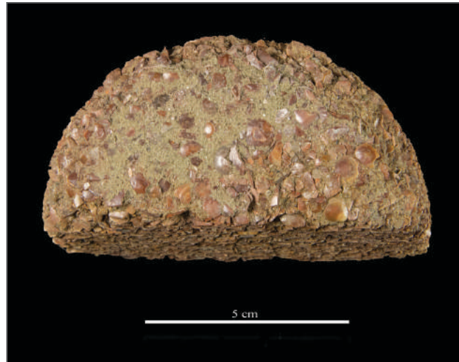
Foto 4.3. Fosforiit (Rakvere; P_2O_5 -sisaldus 6–12%, eU -sisaldus 10–20 mg/kg) Photo 4.3. Phosphorite (Rakvere; P_2O_5 content 6–12%, eU concentration 10–20 mg/kg)
